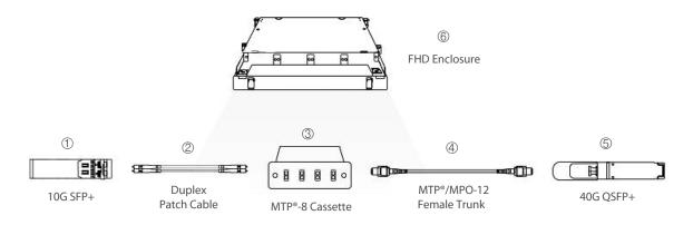
Figure 10: 10G to 40G Inter-connect Connectivity Cabling Utilizing FHD MTP®-8 Cassettes
