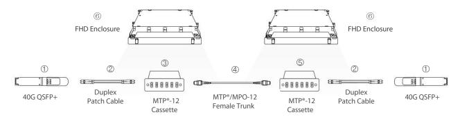
Figure 4: 40G to 40G Inter-connect Cabling with FHD MTP $^{\circ}$ -12 Cassettes
