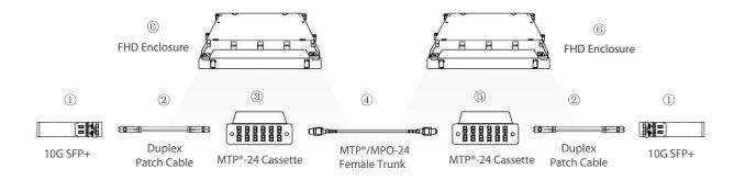
Figure 2: 10G to 10G Inter-connect Cabling with FHD MTP®-24 Cassettes
