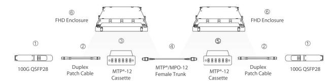
Figure 7: 100G to 100G Inter-connect Cabling with FHD MTP®-12 Cassettes
