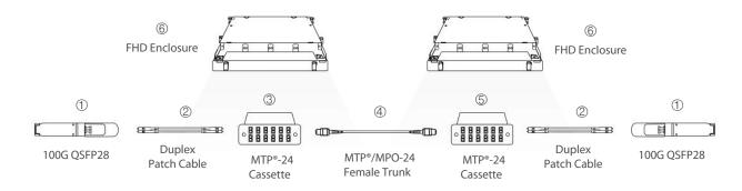
Figure 8: 100G to 100G Inter-connect Cabling with FHD MTP\*-24 Cassettes
