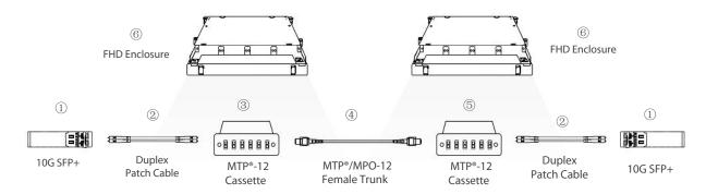
Figure 1: 10G to 10G Inter-connect Cabling with FHD MTP®-12 Cassettes
