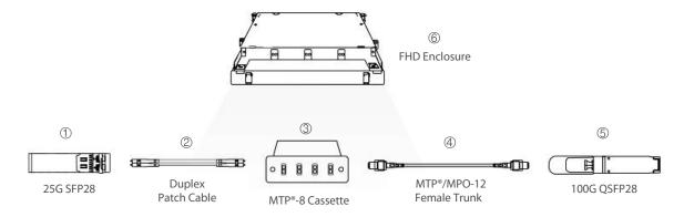
Figure 13: 25G to 100G Inter-connect Connectivity Cabling Utilizing FHD MTP®-8 Cassettes
