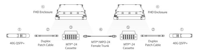
Figure 5: 40G to 40G Inter-connect Cabling with FHD MTP®-24 Cassettes
