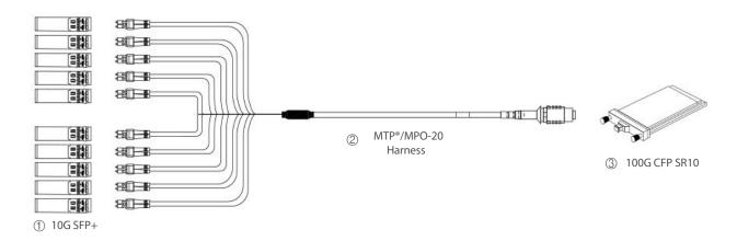
Figure 15: 10G to 100G Direct Connectivity Cabling with a 20-fiber Harness
